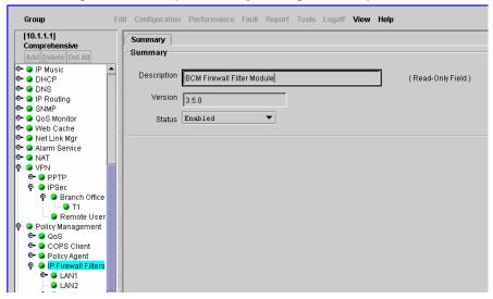
Expand **Policy Management** key, then expand **IP Firewall Filters** Key and click on **LAN2**. The following three rules illustrated on a screen shot below must be configured:
