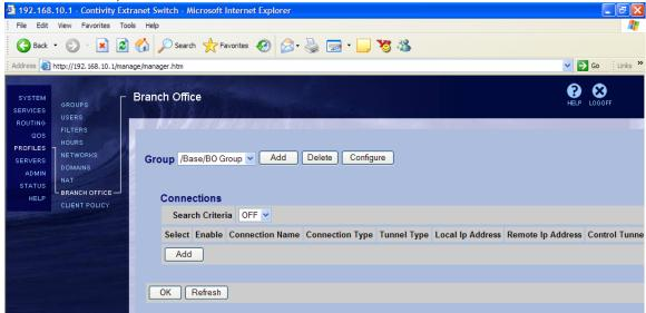
Enter a Connection Name (To BCM), leave the rest of the fields to their defaults – Control Tunnel – Disabled, Tunnel Type – IPSec, Connection Type – Peer to Peer. Click OK: 192.168.10.1 - Contivity Extranet Switch - Microsoft Internet Explorer
